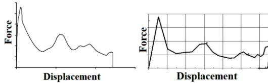
**Fig. 3.3 Force-Displacement characteristics from experiment and simulation**
