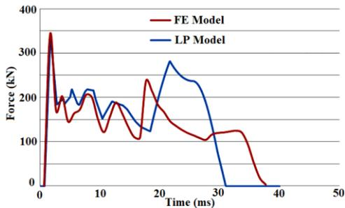
Fig. 4.5 Load history for axial crush of five tubes – FEA and LPM
