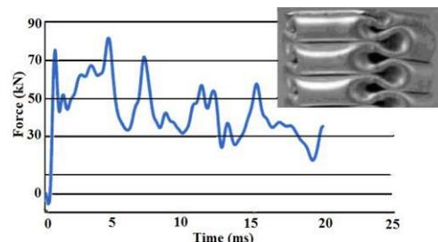
**Fig. 1.1 Progressive buckling failure of a rectangular tube and its Force-Time history**
