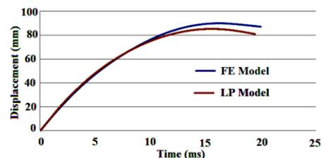
**Fig. 4.3 Displacement - Time history for axial crush of two tubes - FEA and LPM**
