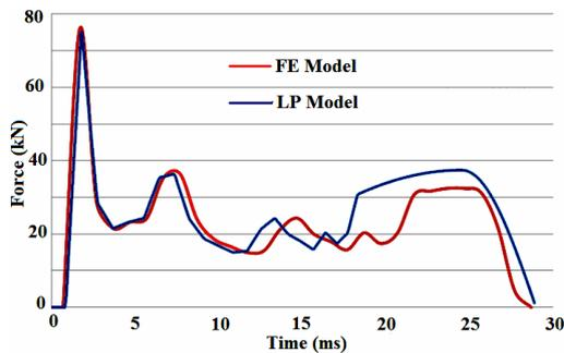
**Fig. 3.4 Force - Time history for axial crush of single tube - FEA and LPM**
