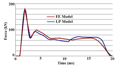
**Fig. 4.2 Force history for axial crush of two tubes - FEA and LPM**
