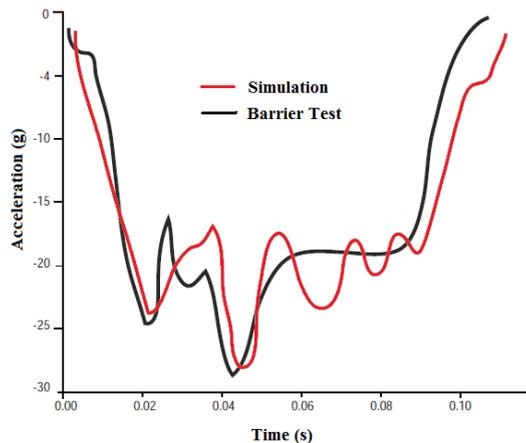
**Fig. 1.2 Crash pulse predicted by LMS model and actual crash test [13]**
