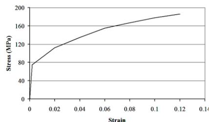
**Fig. 3.2 Stress-Strain curve for A-6060-T4**
