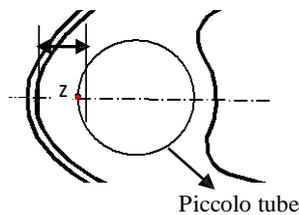
Fig. 7 Distance between piccolo tube and wing inner surface
