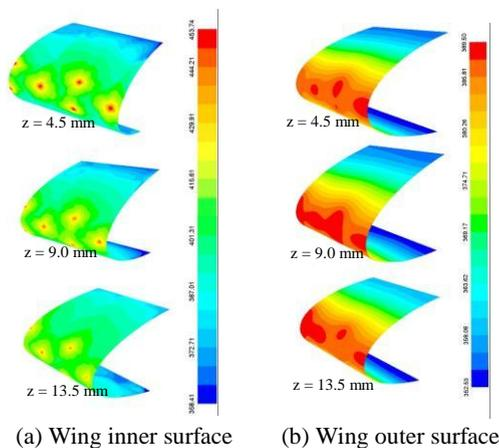
**Fig. 9 Temperature distribution on inner and outer surfaces of the wing for  $z=4.5$ ,  $9.0$  and  $13.5$  mm --- 3D simulations**
