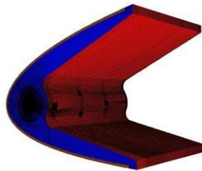
Fig. 6 Discretised 3D flow domain of aircraft wing leading end with piccolo tube
