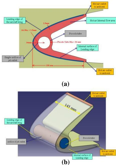
Fig. 3 2D and 3D models of wing and piccolo tube assembly
