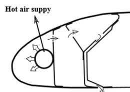
**Fig. 1 A typical thermal anti-icing system using piccolo tube**
