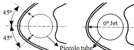
Fig. 4 Angular positions of hot air impinging jets
