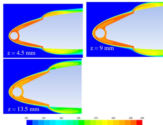
Fig. 8 Total temperature distribution with two jets at +45° and -45° and  $z = 4.5, 9$  and  $13.5$  mm
