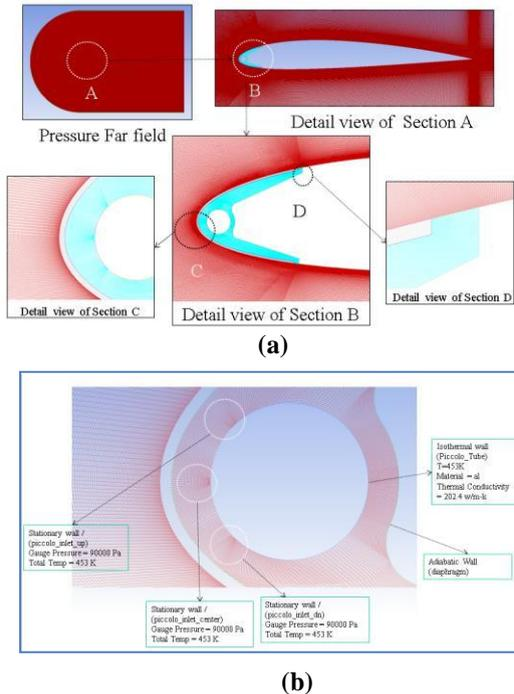
Fig. 5 Discretised 2D flow domain and boundary conditions for NACA 2412 aerofoil
