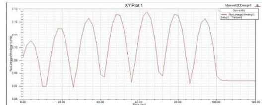
Fig. 6 Flux linkage plot for concept I, case I
