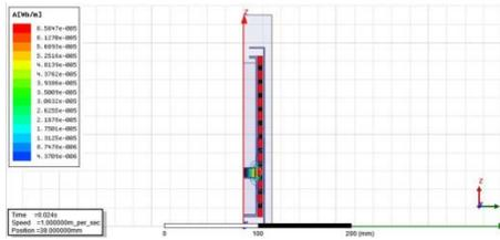
Fig. 8 Flux line plot for concept I, case II
