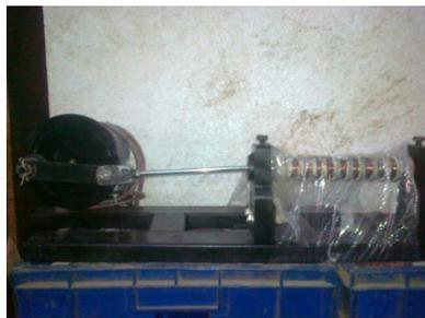
Fig. 4 Fabricated regenerative shock absorber
