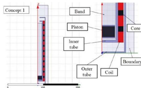
Fig. 2 Concept I finite element model
