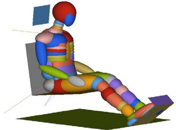
**Fig. 7 Dummy positioned with all the restraint system**
