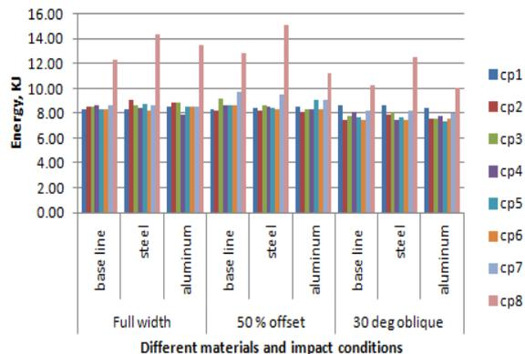
Fig. 12 Energy absorbed by different concepts for different materials and impact conditions
