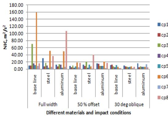
**Fig. 14 Neck injury criteria value for different materials and impact conditions**
