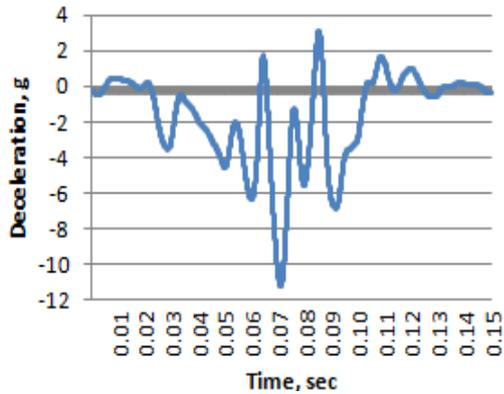
Fig. 11 Deceleration versus time plot for full width impact condition
