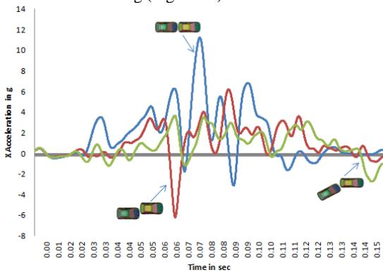
Fig. 10 Crash pulse for different impact conditions
