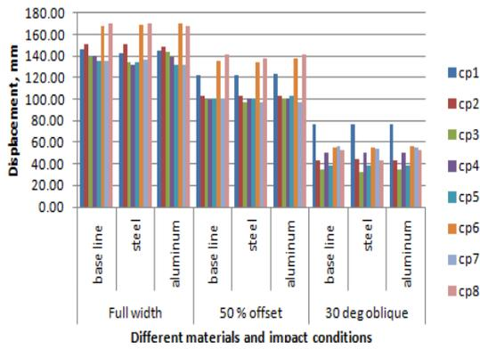
**Fig. 13 Displacement of differnt concepts for different materials and impact conditions**
