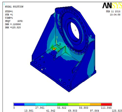
**Fig. 6 von-Mises Stress in Pedestal Existing Design**
