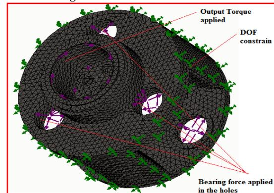
**Fig. 5 Meshed Model of Planet Carrier**
