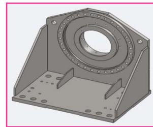
Fig. 3 Pedestal used in Gearbox
