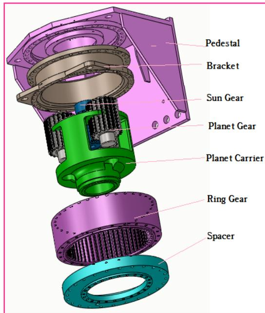
Fig. 1 Exploded View of Gearbox Assembly
