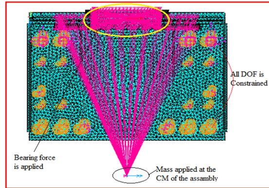
**Fig. 4 Meshed Model of Pedestal**
