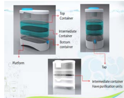
Fig. 25 Concept 3 – Water Purifier
