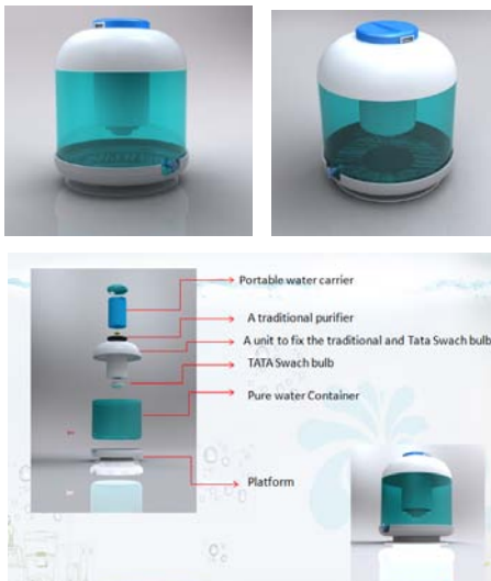
Fig. 23 Concept 1- Water Purifier
