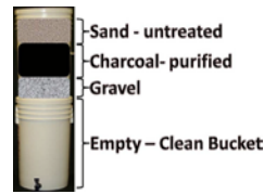
Fig. 5 Water Filtration using Sand and Gravel
