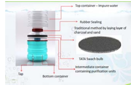
Fig. 24 Concept 2 – Water Purifier
