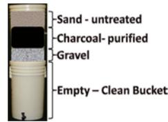
**Fig. 5 Water Filtration using Sand and Gravel**
