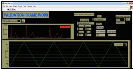
**Fig. 16 Generation of Triangular Waveform**
