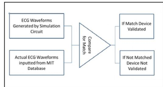
Fig. 2 Design for Generating ECG Waveforms
