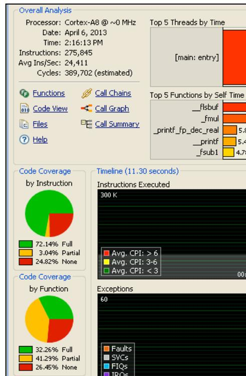
**Fig. 5 RVDS Profiling for ARM Cortex A8**
