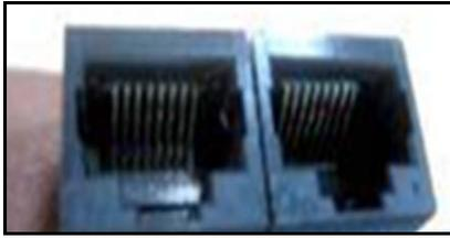
**Fig. 5 Telejack pin corrosion**
