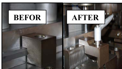
Fig. 9 Improved clamping system using toggle clamps
