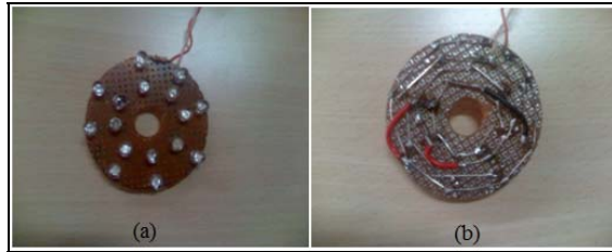
Fig. 3 Concentric arrangements of IR LED's for better illumination (a); parallel connection of IR LED's (b)
