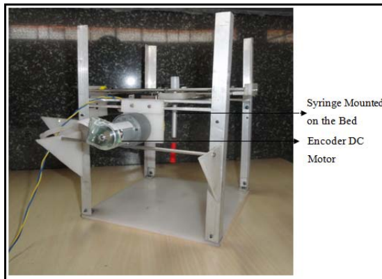
Fig. 16 Figure displaying the device with syringe and the motor
