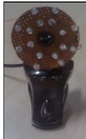
Fig. 4 Imaging device with IR LED arrangement
