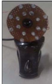
**Fig. 4 Imaging device with IR LED arrangement**
