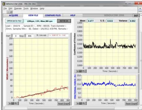
**Fig. 8 Wear, Coefficient of friction, Frictional force versus time for cylindrical particles**
