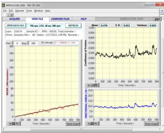
**Fig. 9 Wear, Coefficient of friction, Frictional force versus time for right circular**
