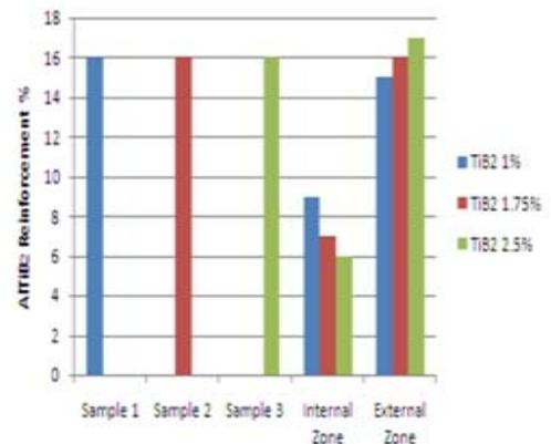
Fig. 3 Measured volume fraction of reinforcement
