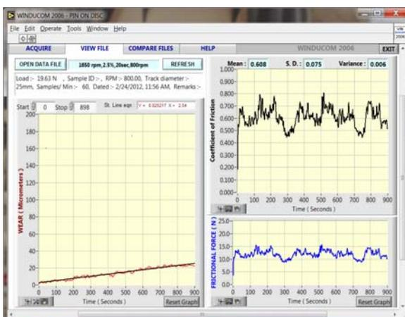
**Fig. 10 Wear, Coefficient of friction, Frictional force versus time for tetrahedron shape particles**
