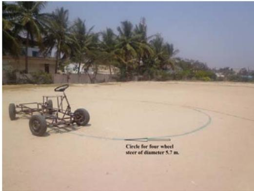
**Fig. 19 Constant radius test conducted for four wheel steer.**
