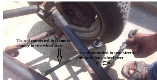
**Fig. 9 Tie rods for converting from four wheel steer to two wheel steer**
