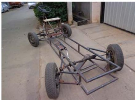
Fig. 12 Four wheel steer of prototype model
