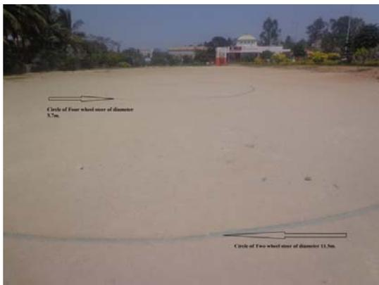
**Fig. 20 Comparison circle of 2WS and 4WS**
