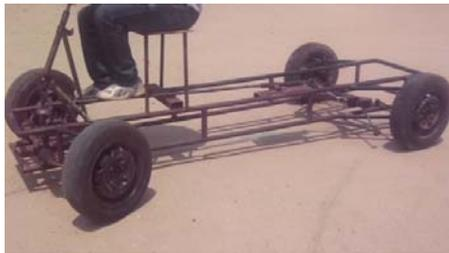
Fig. 11 Two wheel steer of the prototype model
