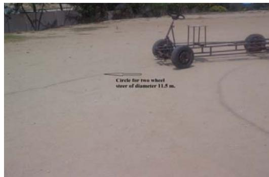
**Fig. 18 Constant radius test conducted for two wheel steer.**
