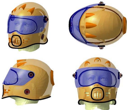
Fig. 4 Ergonomic analysis of helmet with 50th percentile male dummy
