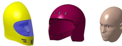
**Fig. 5 Geometric model of Helmet, cushion and head**
