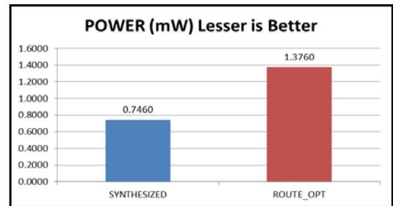
Fig. 8 RTL synthesis and PD Power comparison
