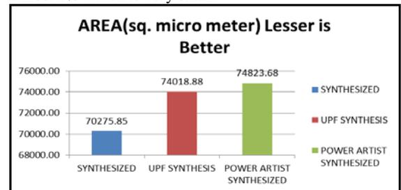
Fig. 5 RTL synthesis design area comparison
