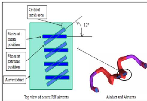
**Fig. 7 Plan view of centre right airvents**
