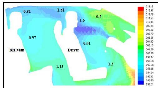
**Fig 15. Driver plane temperature contours with air velocities (m/s)**
