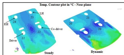
**Fig 16. Nose plane temperature plots for steady and dynamic conditions**
