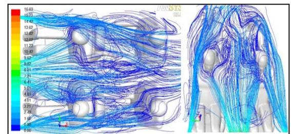
Fig. 13 Airflow directivity with dynamic airvents, 2 cycles
