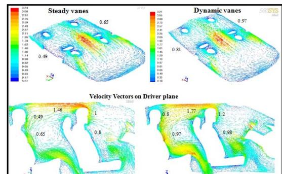
**Fig. 9 Velocity vectors for steady and dynamic airvents at nose and driver planes (Z-Z section)**
