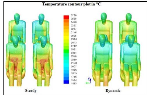
**Fig. 14 Temperature contour plots for steady and dynamic vents case**
