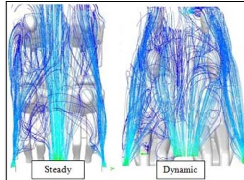
**Fig. 8 Pathlines colored with velocity for dynamic and steady airvents model**
