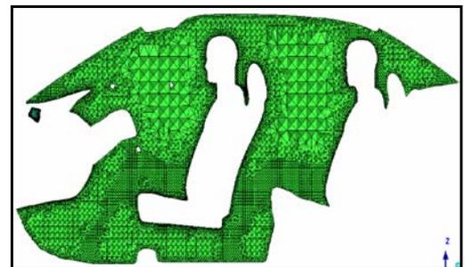
**Fig. 5 Meshed section of cabin**
