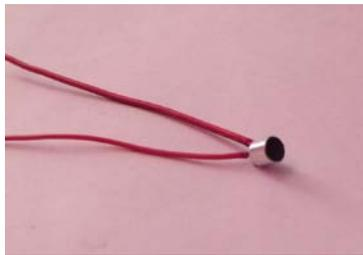
**Fig. 4 Electret Condenser Microphones**
