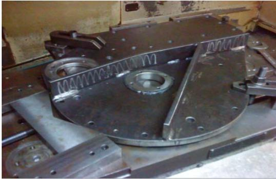
**Fig. 9 Component clamped on fixture**
