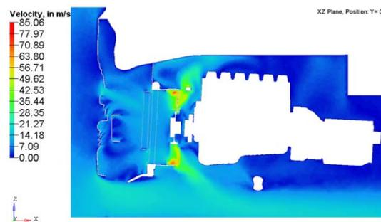
**Fig. 9 Velocity contours plotted at symmetry plane for modified model**
