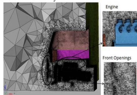
**Fig. 4 Grid generated represented at symmetry plane**
