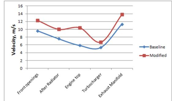
**Fig. 13 Velocity monitored at different locations for baseline and modified model**
