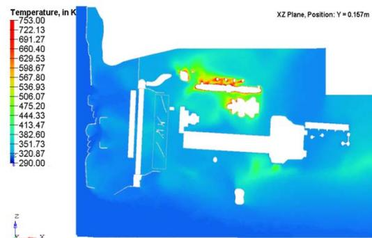
**Fig. 10 Temperature contours plotted at exhaust manifold section for modified model**
