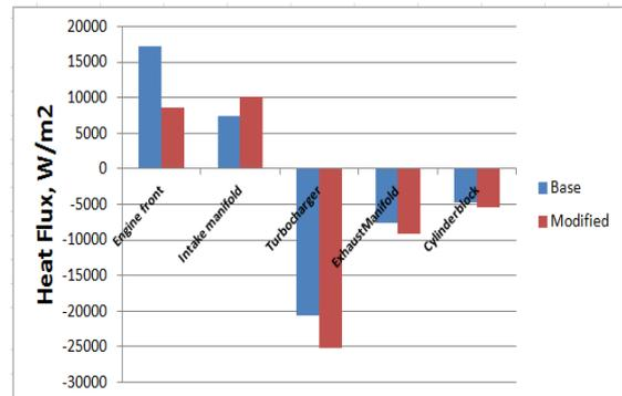
**Fig. 14 Heat flux monitored at different locations for baseline and modified model.**
