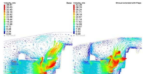
**Fig. 11 Comparison of velocity vectors plotted at radiator section**
