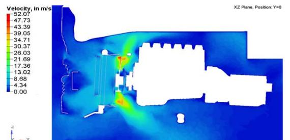
**Fig. 8 Contours colored by velocity magnituded at Maximum torque condition for baseline**
