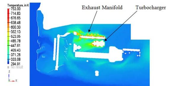
**Fig. 7 Temperature contours plotted at exhaust manifold section for baseline**
