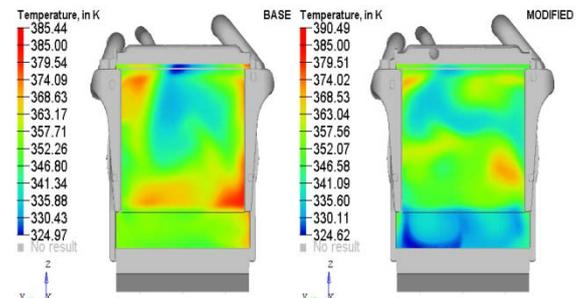
**Fig. 12 Temperature contour plotted on Radiator for baseline (left) with modified model (right)**
