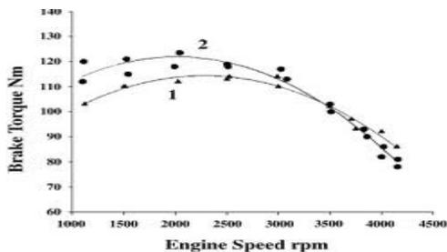
**Fig. 2 Brake torque vs. engine speed curve for trucks** Error! Reference source not found.
