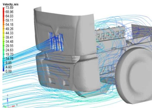
**Fig. 5 Streamlines colored by velocity magnituded for baseline simulation**
