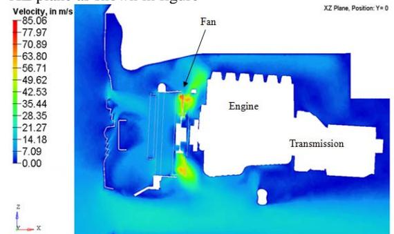
**Fig. 6 Contours colored by velocity magnituded at maximum power condition for baseline**
