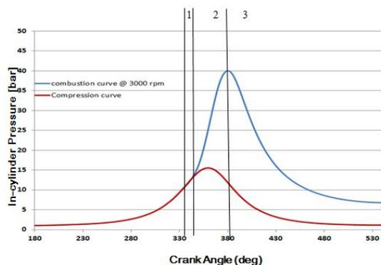
Fig. 7 In cylinder pressure in conventional engine model
