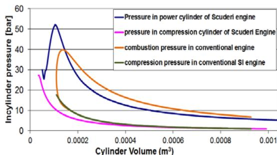
**Fig. 11 p-V curves of conventional engine and Scuderi engine**
