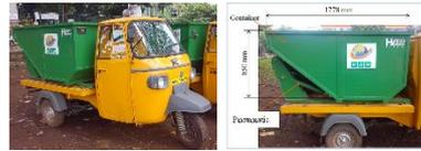
Fig. 4 Dry and wet waste collection vehicle
