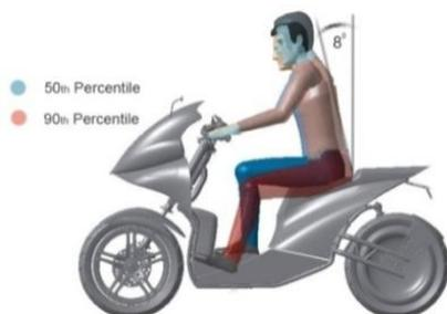
Fig. 10 Ergonomic analysis of final concept
