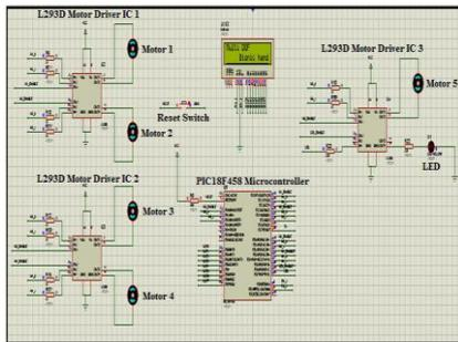
**Fig. 13 Receiver Simulation in Proteus Software**
