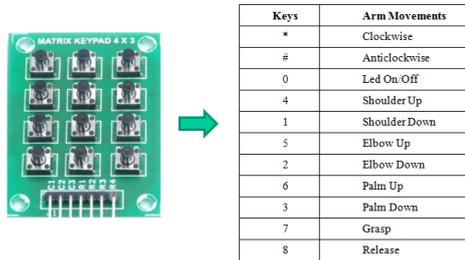
**Fig. 7 Actions Assigned for Keypad Control System**
