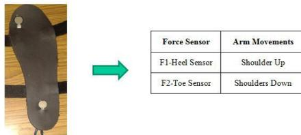
**Fig. 8 Actions Assigned for Foot Pressure Control System**
