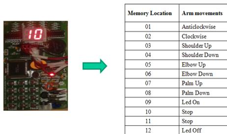
**Fig. 9 Actions Assigned for Speech Recognition Circuit**
