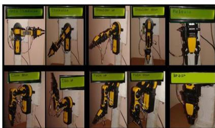
**Fig. 15 DOFs Implemented for OWI Robotic Arm Edge**
