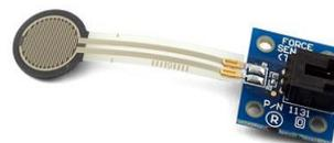
**Fig. 5 Force Sensor used to Control Bionic Arm**
