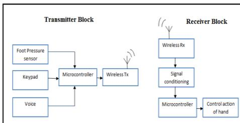
**Fig. 2 Functional Block Diagram of Intelligent Bionic Arm**
