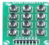
**Fig. 4 Keyboard used to Control Bionic Arm**
