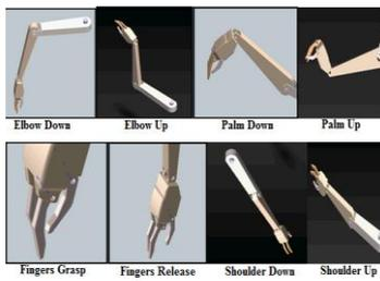
**Fig. 14 Simulated DOFs for Bionic Arm in SolidWork**
