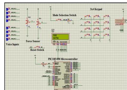
**Fig. 12 Transmitter Simulation in Proteus Software**
