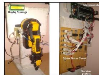
**Fig. 11 Motor Drivers and the OWI Robotic Arm**
