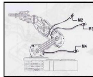
**Fig. 10 Assembled OWI Robotic Arm Edge**
