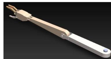
**Fig. 1 Assembled Bionic Arm in CAD Software**
