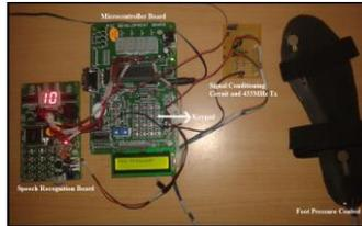
**Fig. 6: Voice Control, Keyboard and Force Sensor Interfaced to Microcontroller**
