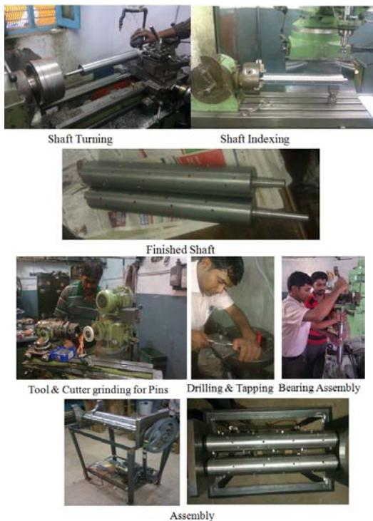
**Fig. 20 Machining and Assembly**
