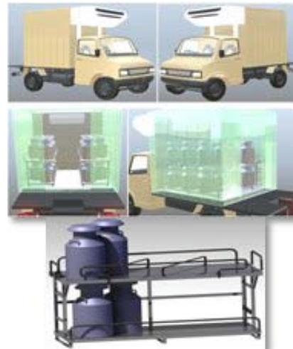
Fig. 15 3D view of Concept-1 of milk van
