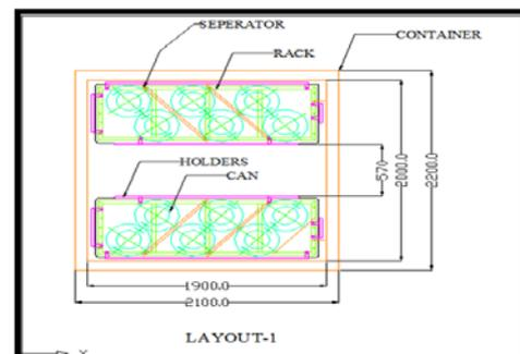
Fig. 12 Interior layout-1 of milk van
