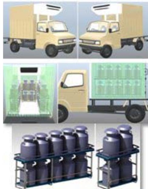
Fig. 16 3D view of Concept-2 of milk van
