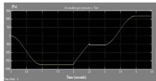
**Fig. 14 Gas pressure variation vs. Time**
