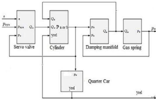
**Fig. 4 Signals and interconnections in the system**
