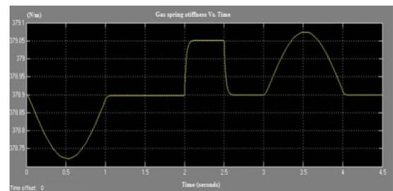
**Fig. 15 Gas spring stiffness vs. Time for hydropneumatic suspension**
