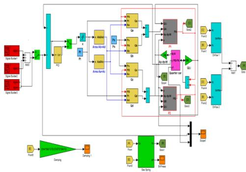
**Fig. 5 Hydropneumatic suspension simulink model**
