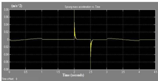
**Fig. 11 Sprung mass acceleration vs. Time of hydropneumatic suspension system**
