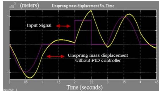
**Fig. 7 Unsprung mass displacement Vs. Time without PID controller**
