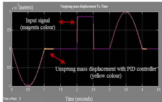
**Fig. 8 Unsprung mass displacement Vs. Time with PID controller**
