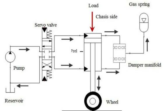
Fig. 1 Hydropneumatic suspension system setup
