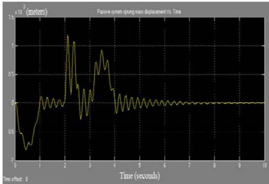
**Fig. 10 Passive system sprung mass displacement vs. Time**
