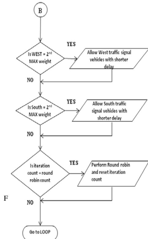
Fig. 6d Block Diagram of Master Node
