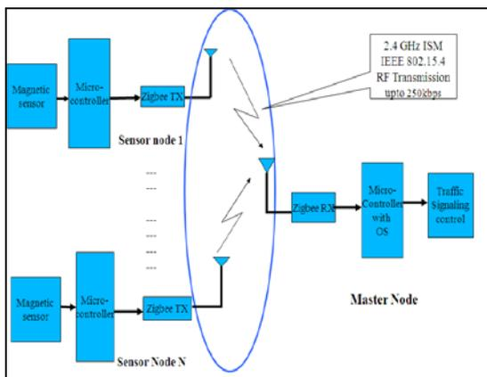
**Fig. 3 Block Diagram of Traffic Monitoring System**
