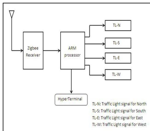
**Fig. 5 Block Diagram of Master Node**
