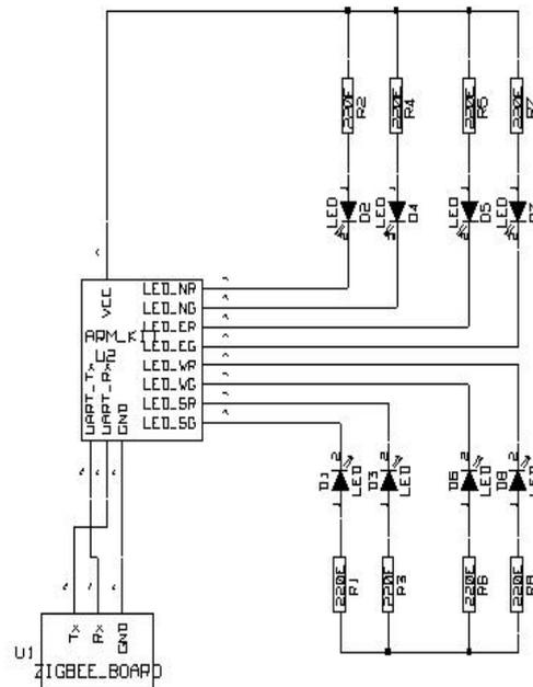
**Fig. 10 Schematic Circuit Diagram for Master Node**
