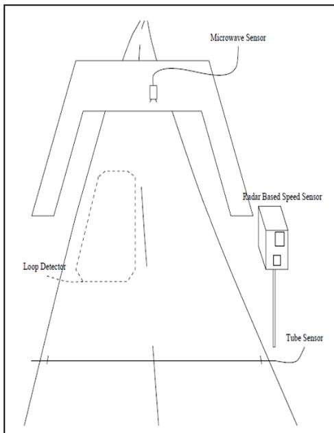
**Fig. 1 Sensors Used for Road-Traffic Monitoring [1]**
