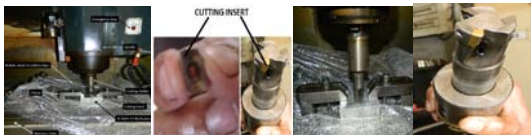
Fig. 7 Set-up for chip morphology study on experimental result
