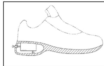
Fig. 3 Electricity Producing Shoe [4]
