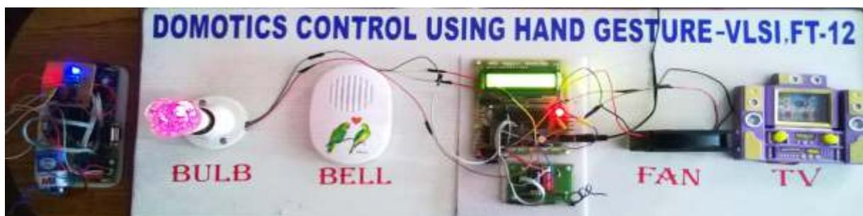
**Prototype model of hand gesture based domotics control system**
