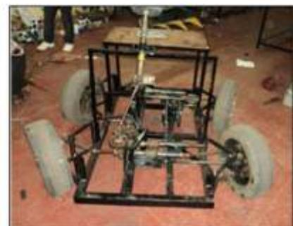
**Development stages of All Wheel Steer Platform: Virtual model and its construction**
