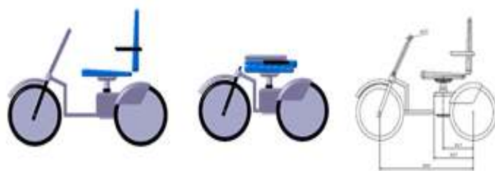
Expanded and collapsed view with dimensions
