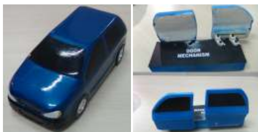
Final mock up model with sliding door mechanism
