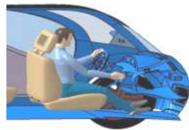
Reach analysis for the driving controls inside the car cabin
