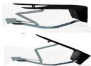
Boot-lid mechanism in closed and open condition
