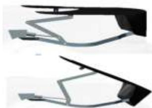
**Boot-lid mechanism in closed and open condition**
