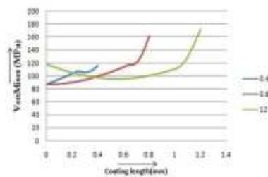
**Von-Mises stress distribution in axial direction**
