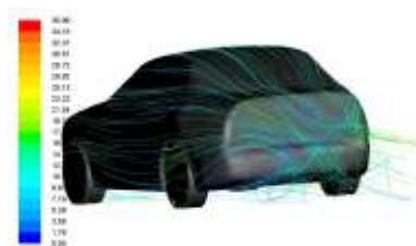
Pathlines coloured by velocity magnitude shown in the wake region for a single car
