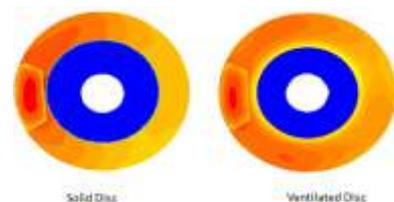
**Comparison of temperature distributions of solid disc and ventilated disc rotors**
