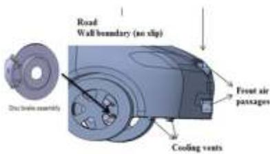
**Disc brake assembly and air intake passages**
