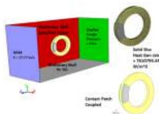
**Boundary conditions for the conjugate heat-transfer on the disc brake assembly**
