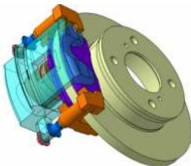
**Disc brake geometric model**
