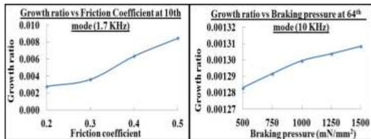
**Effect of friction and braking pressure on squeal characteristics**
