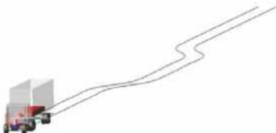
**Path traced by truck semi-trailer during double lane change event**
