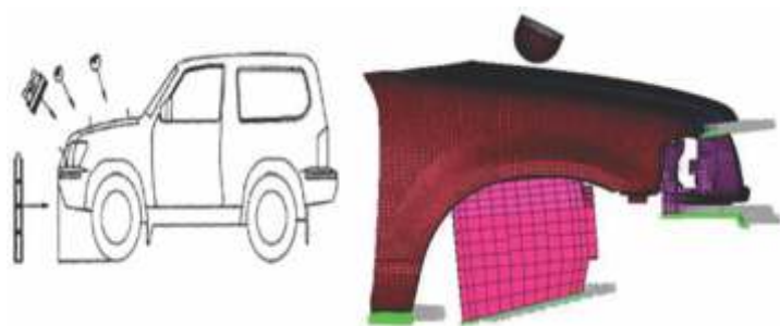
Pedestrian head impact test on bonnet as per EEVC WG17 norms
