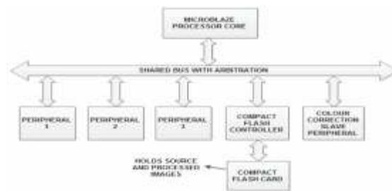
**Colour correction logic as a slave peripheral**
