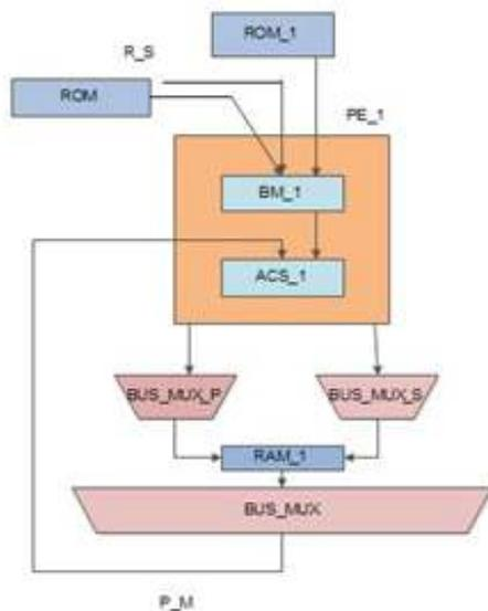
**Systolic architectural design of single processing element of Viterbi decoder**
