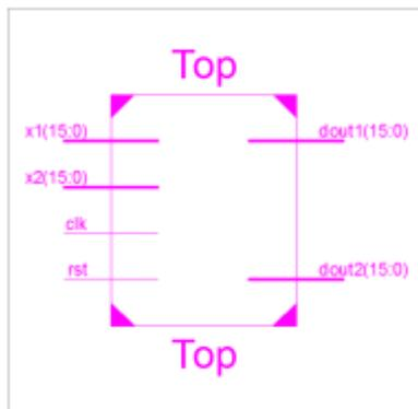
**Top level RTL schematic for STBC encoder**
