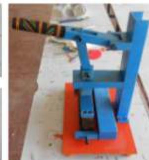
**Prototype of sheet metal bending machine showing portability and easy to assembly of**
