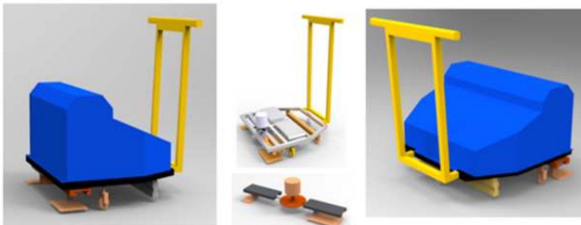
Finalised concept of mechanised floor cleaning device
