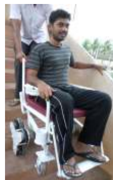
Stair climbing wheel chair - working model in 1:1 scale
