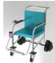
Stair climbing wheel chair shows adjustable foot rest, patient document box, glucose holding stand and calling bell features
