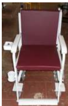
Stair climbing wheel chair - working model in 1:1 scale
