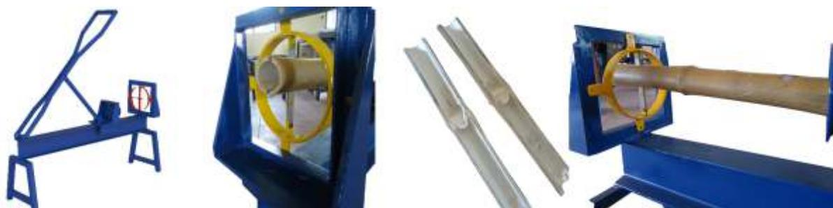
**1:1 working model of bamboo splitting equipments**
