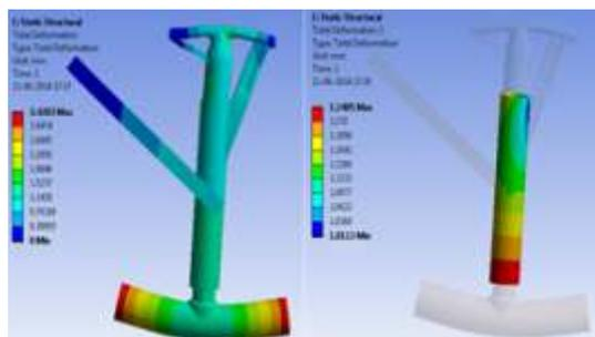
**Deformation plot with [0/90/45/90]s Ti/SiC strut**
