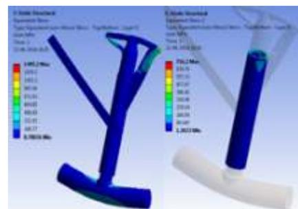
**Stress plot with [0/90/45/90]s Ti/SiC strut**
