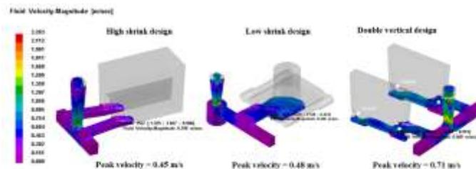
**Simulation of ASTM B208 casting test coupon**
